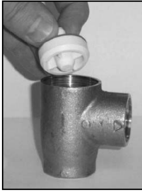
Removing the plunger
