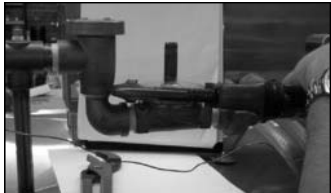
Loosening the valve bonnet
