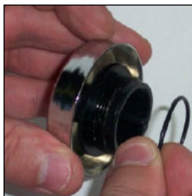
Replacing the O-ring
