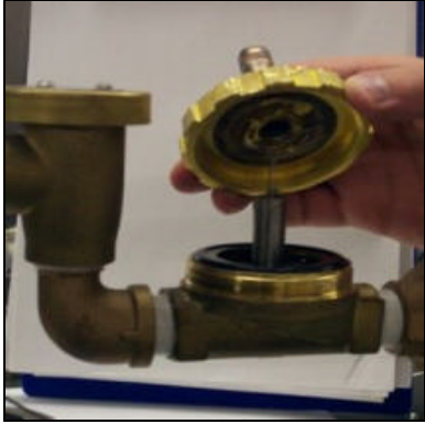
Removing the valve bonnet
