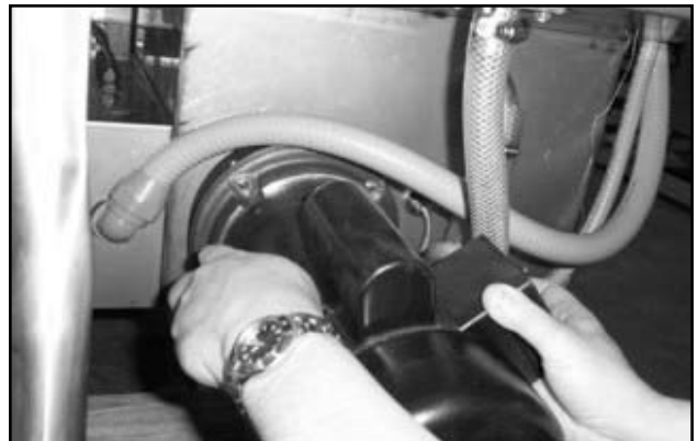
Remounting the wash motor assembly
