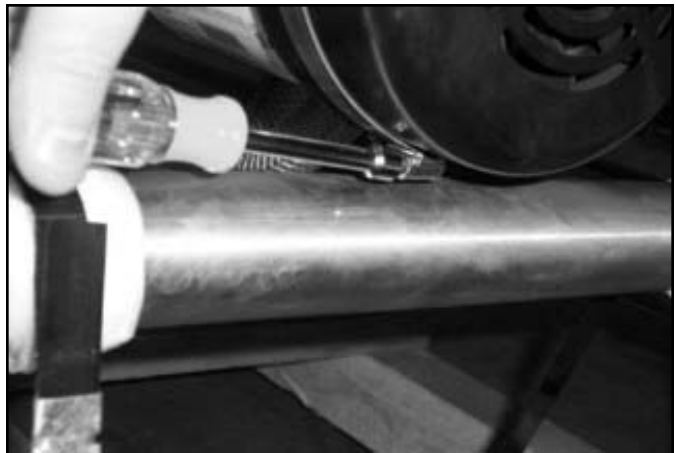
Loosening the band clamp on the back end of the motor.
