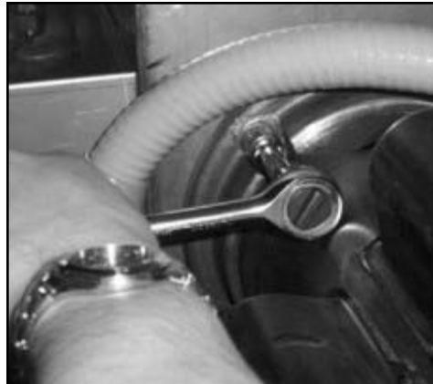
Removing the mounting plate nuts with the 9/16" socket
