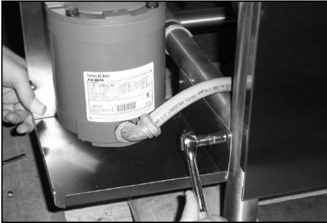
Removing the nuts securing the bottom cover.
