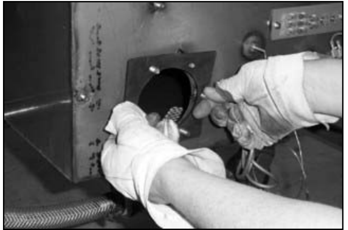
Removing the gasket
