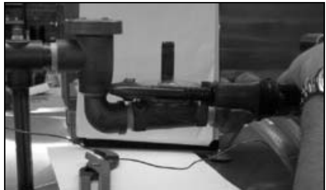
Loosening the valve bonnet
