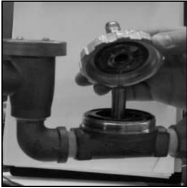
Removing the valve bonnet
