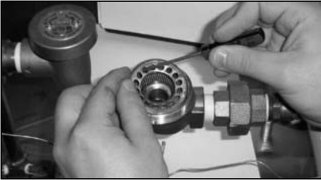
Removing the screen retainer
